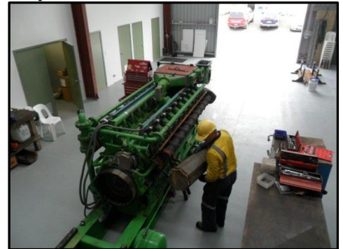
The engine is disassembled, the intake and exhaust manifolds, water rails, water pump, starter motor, oil cooler and electrical components are removed.
