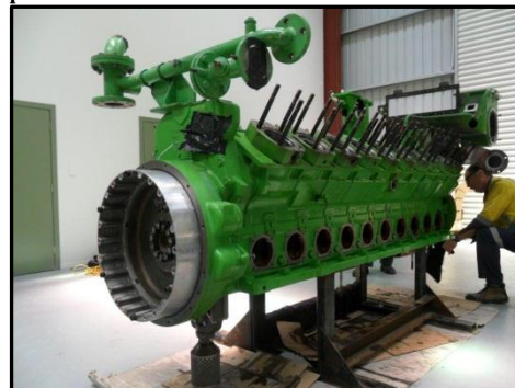
New liners, pistons, big end bearings, piston pins and cam followers are fitted.
